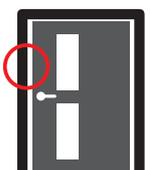
**Intumescent materials** are designed to swell and enlarge when exposed to heat, thereby sealing any gaps in and around a fire door, blocking the path of the fire. Intumescent fire seals are required around the edges of the door – though can be applied to the frame instead.
